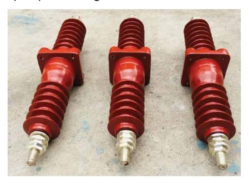
Epoxy bushings are commonly used in transformer manufacturing for their excellent insulating properties and durability. Epoxy bushings have an insulating core made of epoxy resin. Unlike traditional porcelain bushings, epoxy bushings are lightweight and resistant to cracking due to thermal shock
